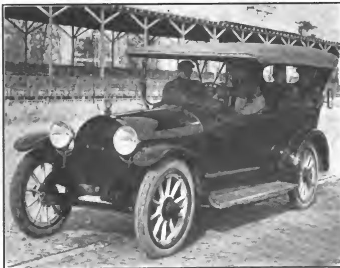
Marmon 41 stock touring car which made 62.89 miles in 1 hour in official tests held at Indianapolis Speedway. Note five passengers and top and windshield raised
